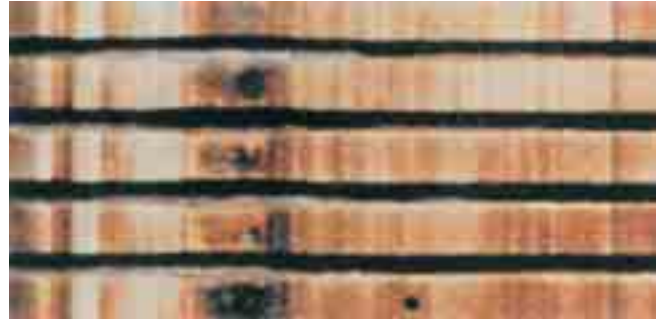
Commutator attack coupled with grooves and burn marks
