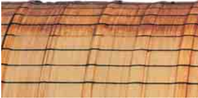
Relatively strong commutator attack with build-up of wear bands and burn ridge formation
