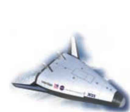
Nose cap with Schunk coating for the space glider CRV. This coating allows for 120 re-entries into the earth's atmosphere.
